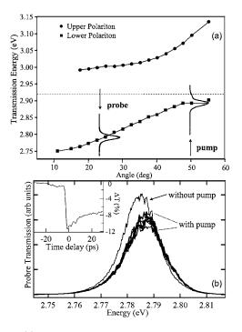
FIG. 3. (a) Pumping away from the magic angle into the excitons. (b) Transmitted probe spectra without the pump pulse and with pump pulse at time delays -10, -5, 0, 1, 3, 5, 10, 20 ps. Inset: time-resolved probe transmission.
