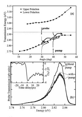
FIG. 2. (a) Angular dispersion of porphyrin microcavity, and pump and probe transmitted spectra at the angles indicated. (b) Transmitted probe spectra (resonantly tuned to the lower polariton dispersion) without the pump pulse and with pump pulse at time delays -10, -5, 0, 1, 3, 5, 10, 20 ps. Inset: time-resolved probe transmission at 2.83 eV.
