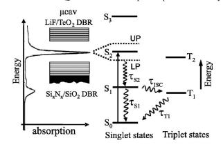
FIG. 1. Absorption spectra of zinc porphyrin dye and corresponding energy states  $S_n$  singlets,  $T_n$  triplets. Microcavity is formed by positioning the organic film between two dielectric mirrors. Two new states LP, UP separated by Rabi energy are formed through resonant light–matter interaction.
